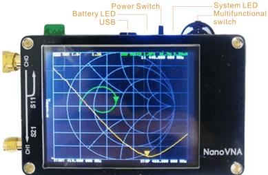
You can use the USB interface to connect to computer communications or connect standard 5V charger charging.
